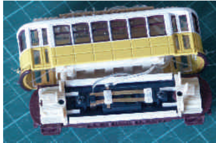
photo 3 Kato chassis in place
